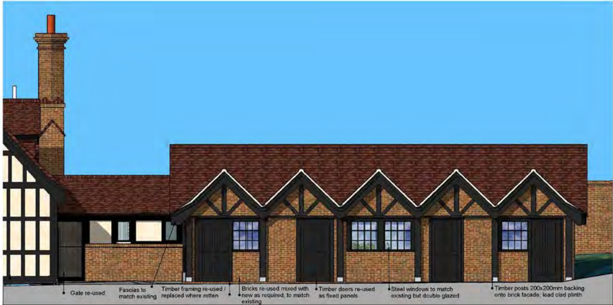
East elevation proposed with gables raised to match pre-existing conjecture prior to subsidence Railings removed for clarity Refer to 212_21
