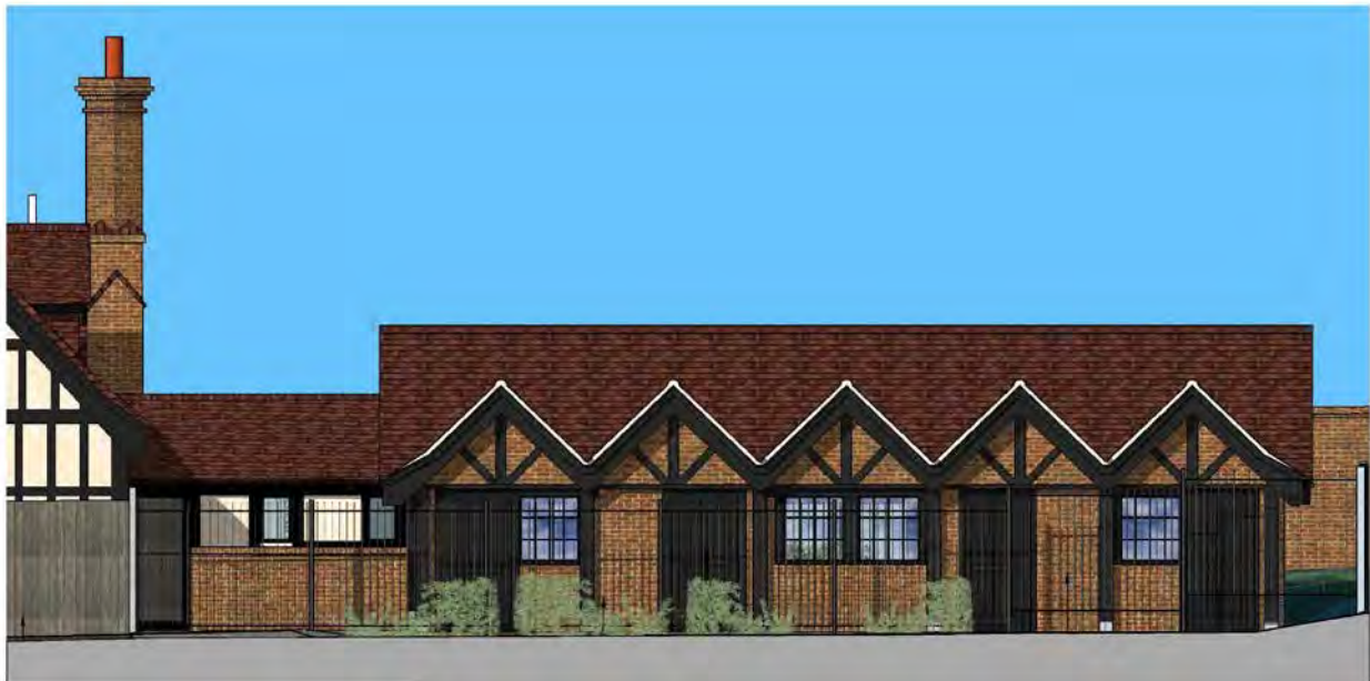
East elevation proposed with gables raised to match pre-existing conjecture prior to subsidence
